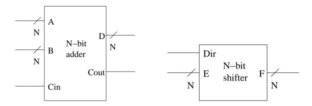
The N-bit adder takes three inputs A, B, and  $C_{in}$ , and produces two outputs D and  $C_{out}$ .
