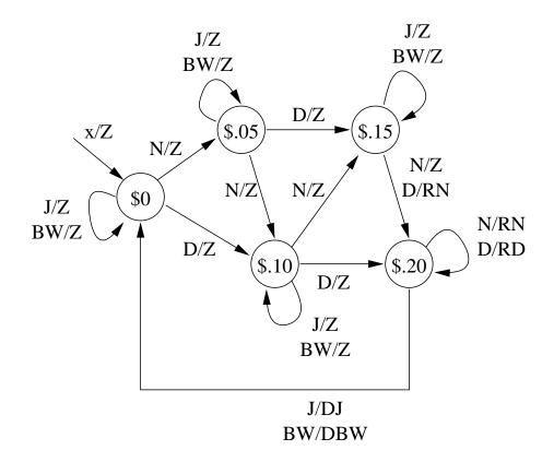
Where the events are: N = Nickel (insertion); D = Dime (insertion); J = Jolt (request); BW = Buzz Water (request).
