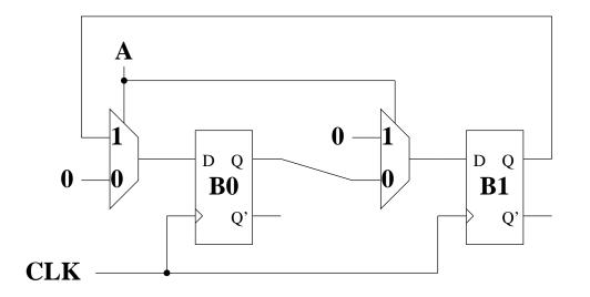
(a) (6 pts) Assume that the initial state is B1 = 0 and B0 = 1, and that A = 0. Fill in the following timing diagram:
