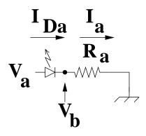
Assume  $R_a = 500\Omega$  and  $V_{fa} = 3V$ .
