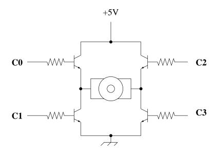
(5 points) What configuration of C signals would result in a dynamic braking of the motor?
