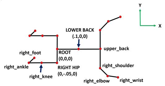
The root of our kinematic tree is located at the origin of our three dimensional space (x = 0; y = 0; z = 0). This root point is connected to three other points through fixed relationships: the *lower back* is always located at x = 0.1; y = 0; z = 0, and the left and right hip socket joints are located at x = 0; y = 0.05; z = 0 and x = 0; y = -0.05; z = 0, respectively. We refer to these three points as the *children* of the root point.
